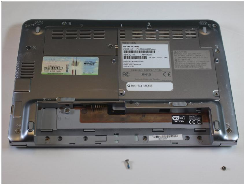
*(i)* Note that the screw on the left is longer than the screw on the right.
