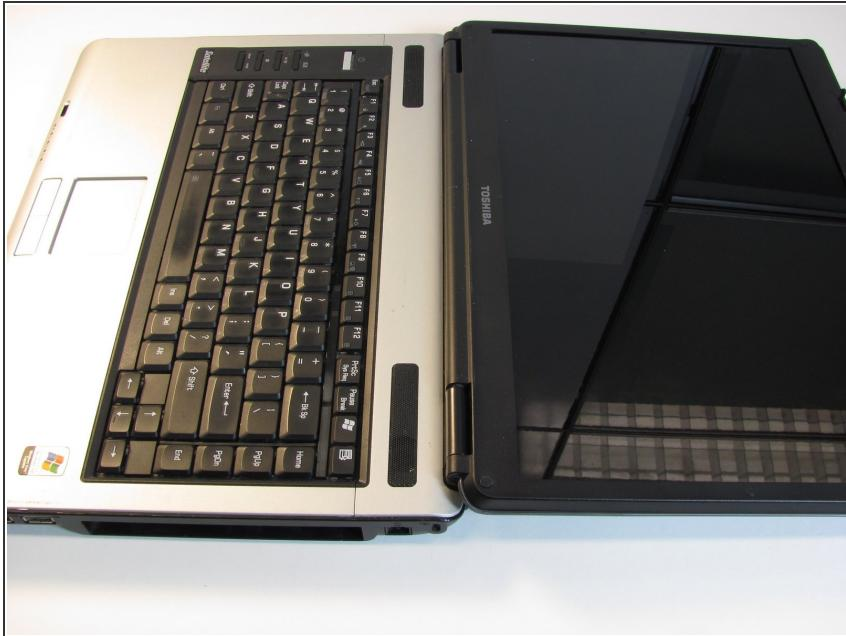
*(i)* Flip the laptop over so it is rightside up, and open the laptop all the way so that the screen is horizontal.
