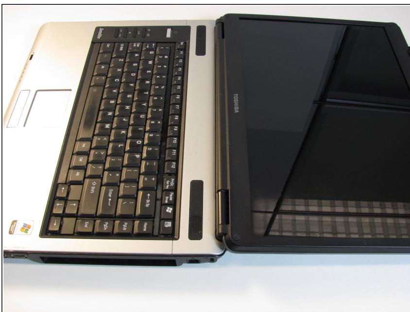
i Flip the laptop over so it is rightside up, and open the laptop all the way so that the screen is horizontal.
