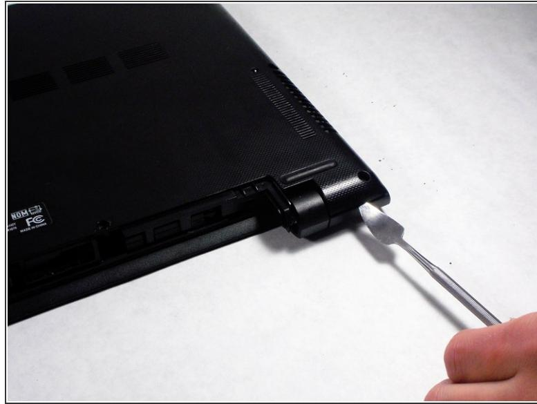
! Using a metal spudger can damage sensitive components.
