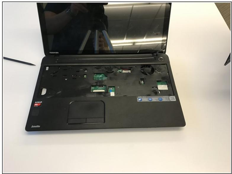
⚠ Before pulling out the keyboard, notice that it is connected to the motherboard via a ribbon cable. Gently press out the ribbon cable from its connection site and put the old keyboard aside.
