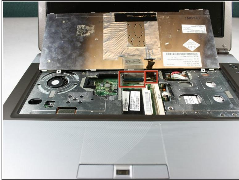
**⚠** When removing the keyboard, be careful not to rip the ribbon cable connecting the keyboard to the computer, to avoid damaging it.
