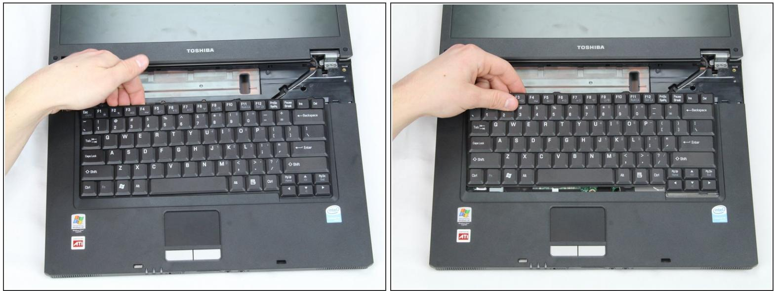
**⚠** There is a ribbon cable underneath the keyboard. Don't lift the keyboard too forcefully or you may break the ribbon cable.
