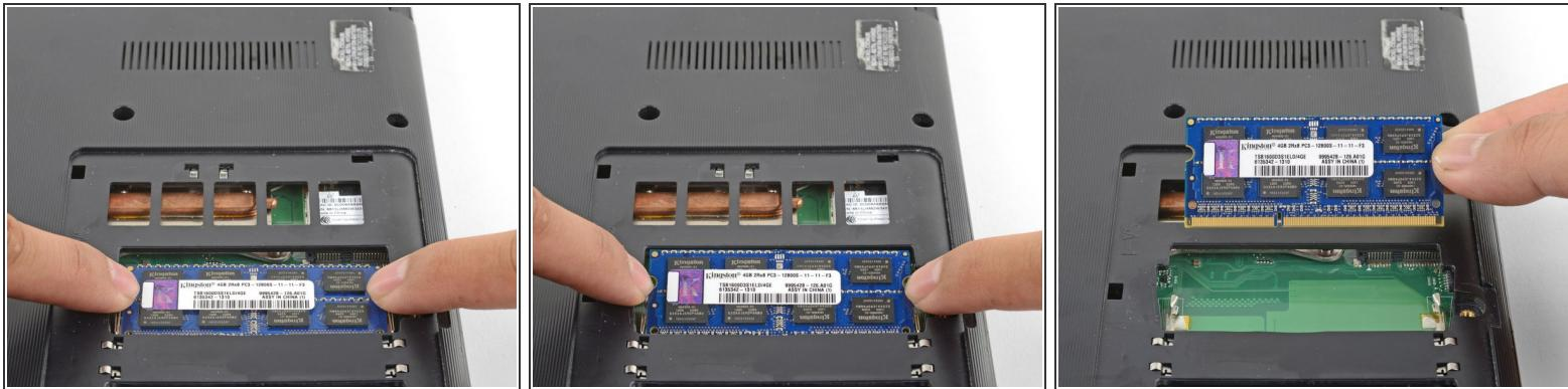
*(i)* This step shows how to remove a RAM module.
