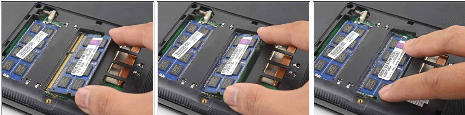
*(i)* This step shows how to insert a RAM module.
