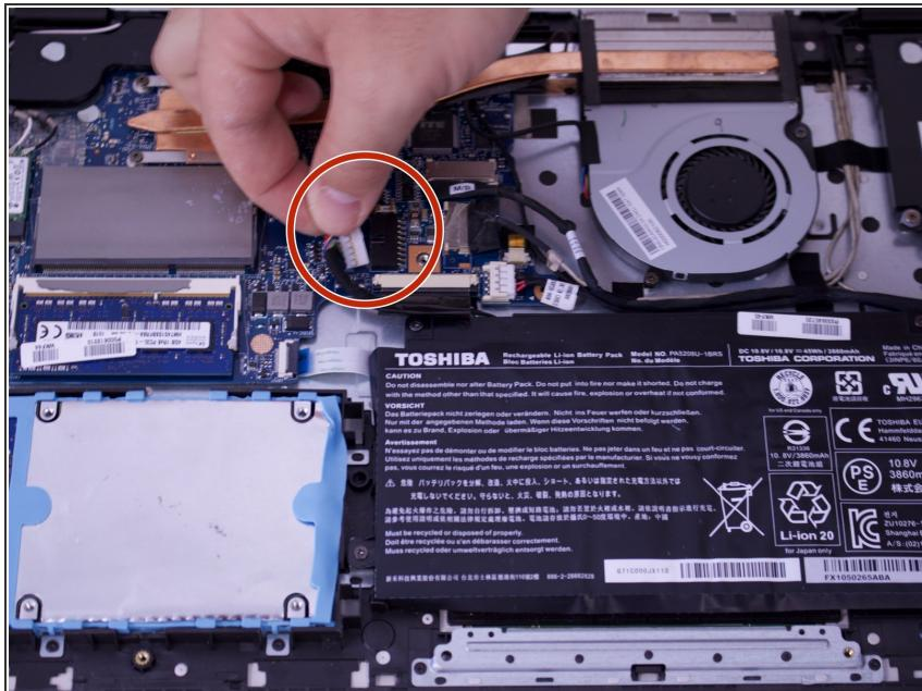
**!** Before touching any component inside your device, ensure you are properly grounded with an anti-static band.
