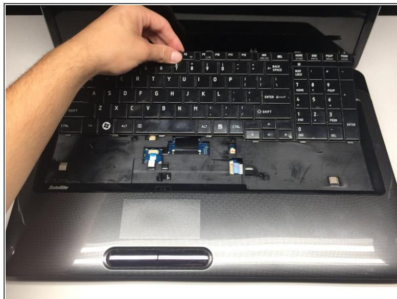
**⚠** Lift the keyboard gently . Slide it forward towards the screen and speakers. This reveals the connection needed for the next step.
