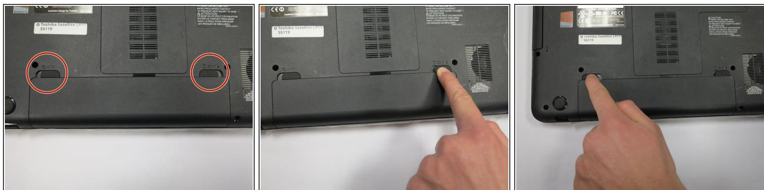
**①** Locate the battery latches. The battery latch mechanism can be compared to a door -- The right latch, when pushed right, unlocks the battery, while the left latch, when pushed left, releases the battery, pushing it out from its container.
