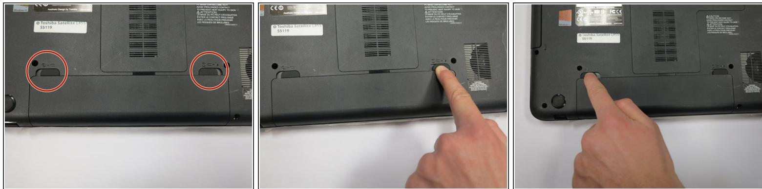
*(i)* Locate the battery latches. The battery latch mechanism can be compared to a door -- The right latch, when pushed right, unlocks the battery, while the left latch, when pushed left, releases the battery, pushing it out from its container.
