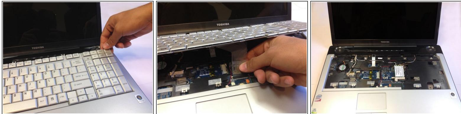
**⚠** Be careful to not lift up on the keyboard too quickly or harshly; there is a ribbon cable connecting the keyboard and the base which may be breakable.
