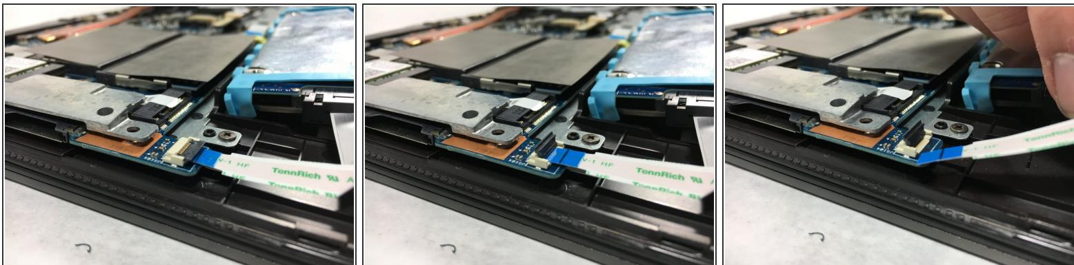
⚠ Do not pull on the ZIF connector that connects the hard drive to the laptop.
