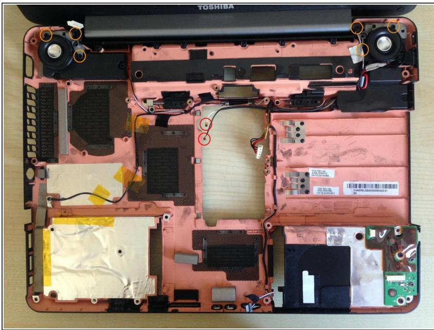
**⚠** Before attempting to remove the screen or any other components left in the shell, make a careful note of how each cable is routed. Take detailed photos if your laptop is not identical to this one.
