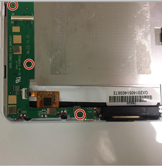
*(i)* The smaller portion of the motherboard is located at the bottom with the speaker.
