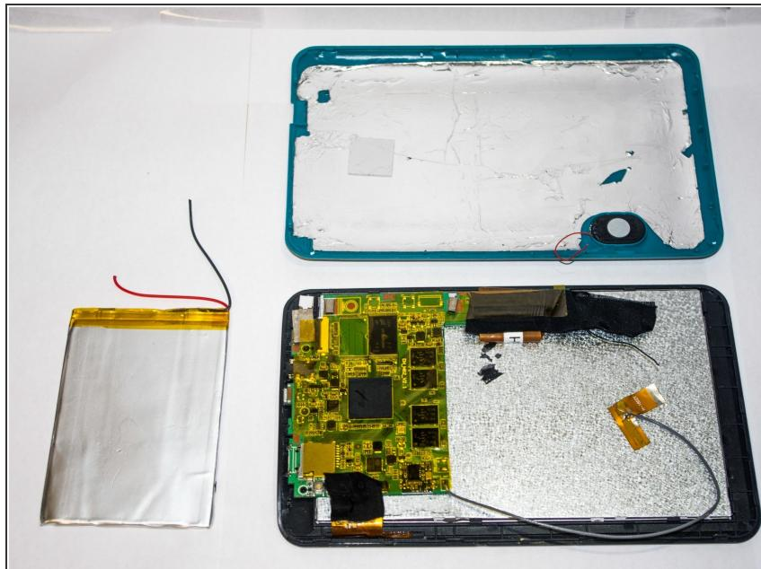
**!** In order to replace the battery once the wires are removed, you will need to solder the wires of the new battery onto the motherboard.
