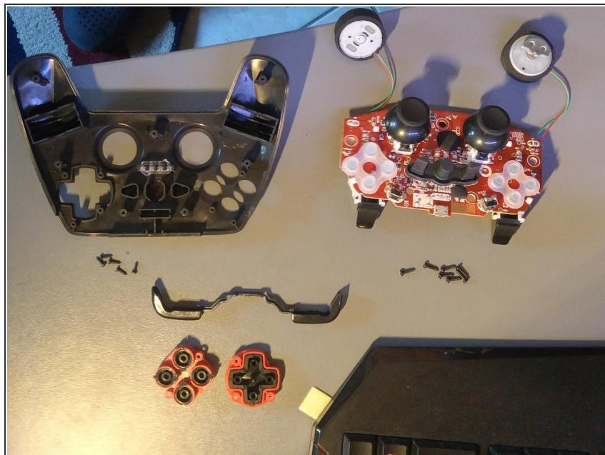
*(i)* You now have a fully disassembled controller, ready to be repaired or modified
