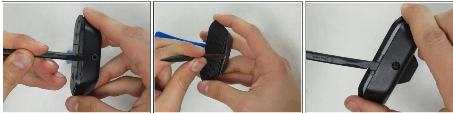
**⚠** Be firm but controlled with the [Spudger](#). Excessive force may cause tool marks or crack the plastic causing structural damage.
