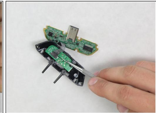
**⚠ Handle with care. The wires and the traces on the circuit board break easily.**
