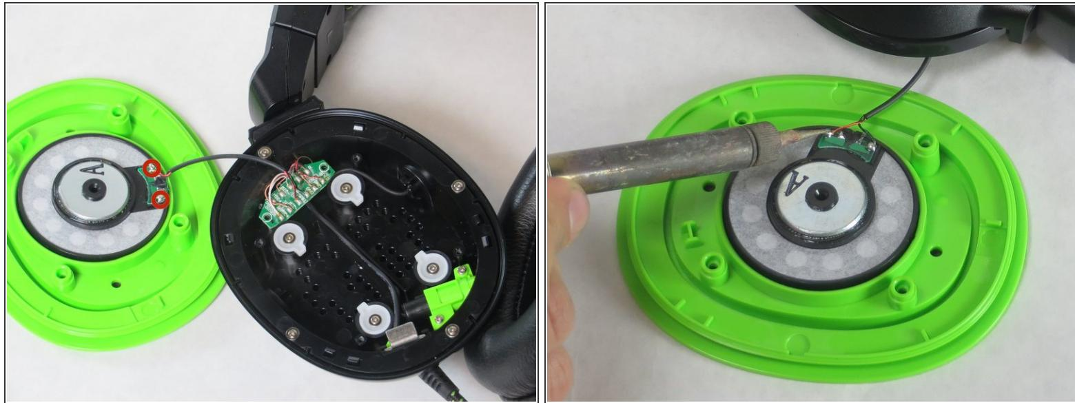
**⚠** When removing the speaker cone plate, be careful not to drop it or put stress on the wires as they are very delicate.
