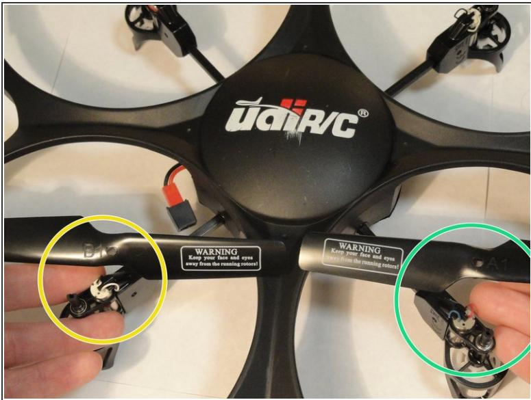
*(i)* Motor direction and propeller direction is crucial to proper flight, refer to this format.
