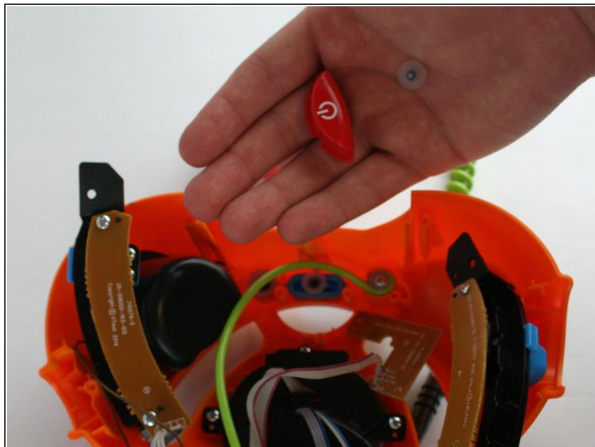
⚠ Carefully move the power button board out of the way.
