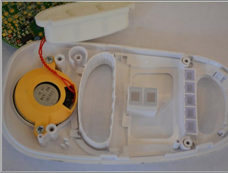
**⚠** When separating the motherboard from the front cover, be careful not to disconnect the two red wires which connect the speaker to the motherboard.
