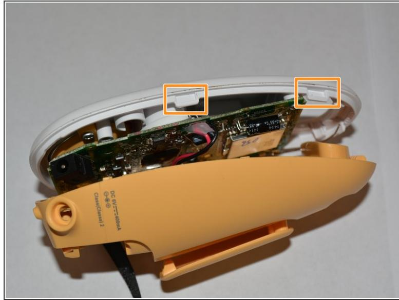
ⓘ The white front covering of the device is held to the yellow back covering by four clips on the back covering which fit into tabs on the front covering.
