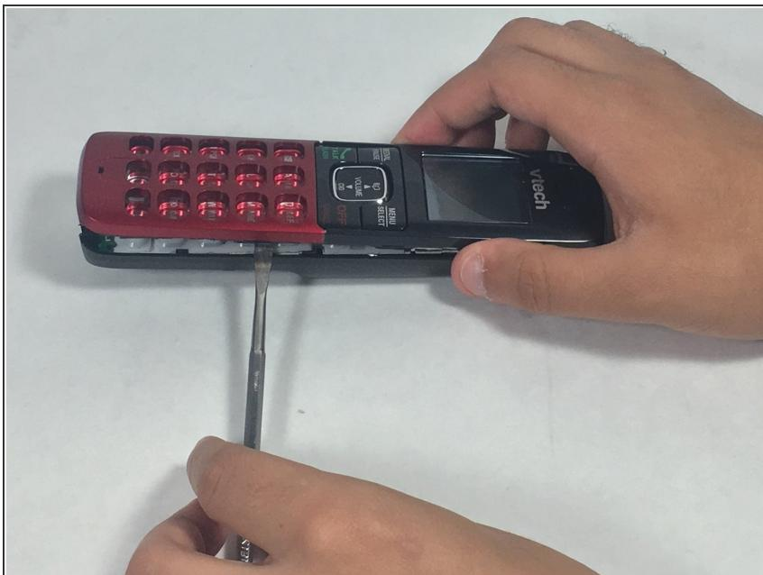
⚠ After removing the two screws from the back of the phone carefully use the metal spudger to lift along the edges and raise the phone case from the internal clips.
