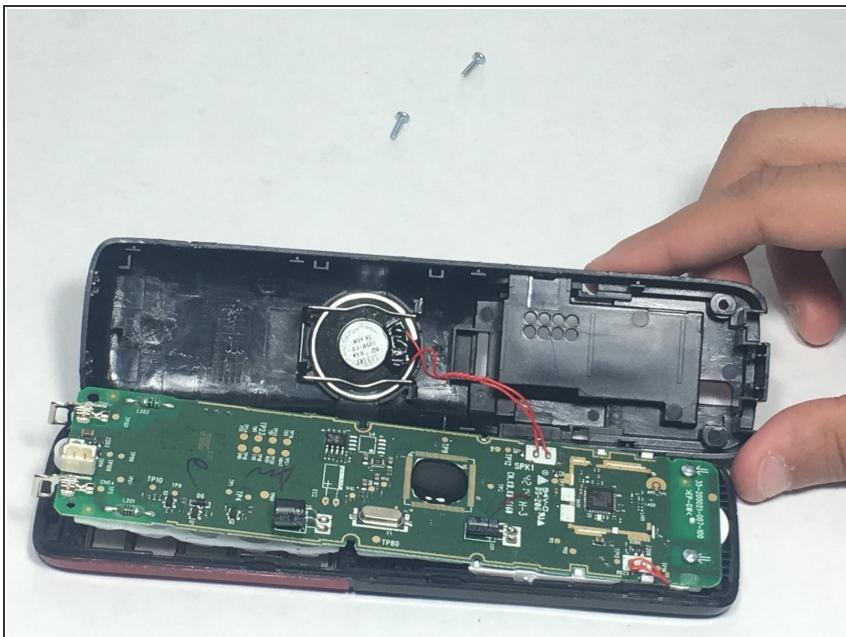
ⓘ Once the case is lifted, the board should be freed except for the connection between the ringer and the case.
