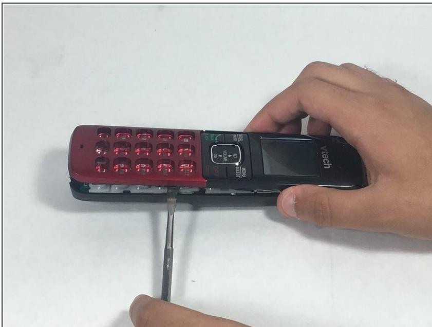
**⚠** Using the metal spudger gently, but firmly edge along the device .
