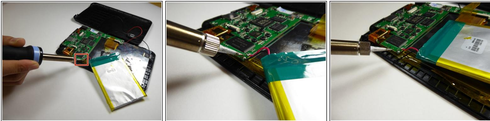
**⚠** Soldering iron gets hot. For information on how to use a soldering iron, click [here](#).
