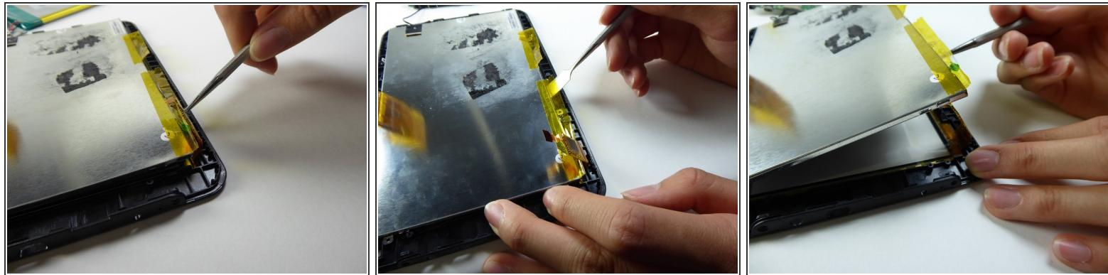
! Be careful on this step - the screen is fragile and can break easily.
