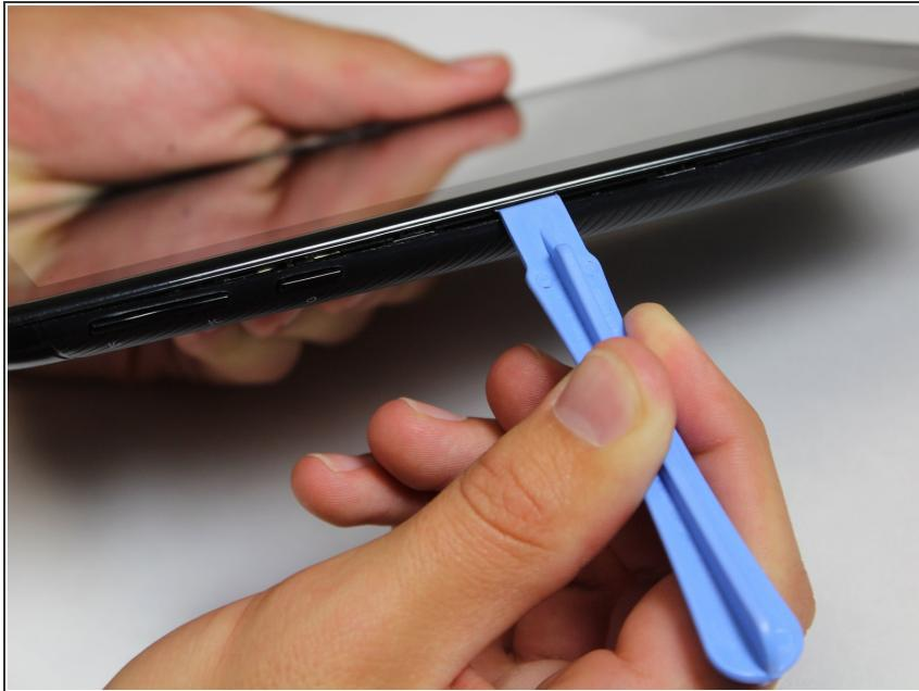
**⚠** Be careful when taking the back panel off. The speaker is connected to both the front and back panels, and may get pulled out if you are not gentle when lifting the back panel away.
