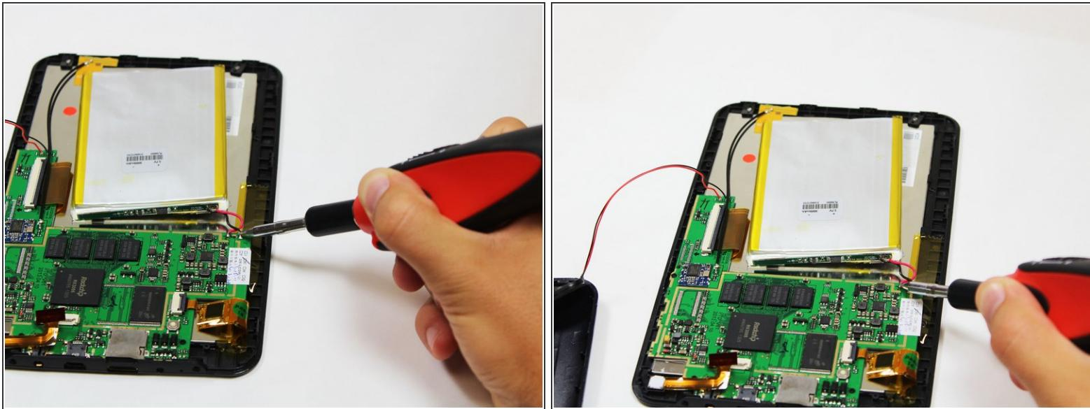
⚠ Soldering guns are hot and can easily damage the device.
