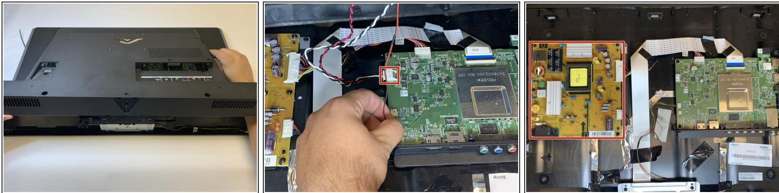
⚠ There are two speaker wires attached to the back of the TV Panel.
