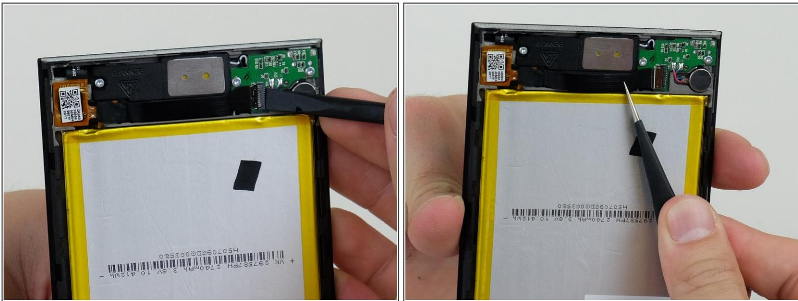
⚠ The black ribbon can be easily damaged during this step, so proceed with caution.
