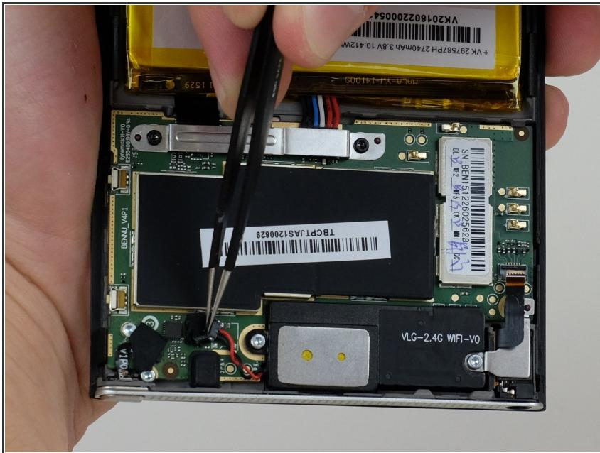
⚠ During this step, avoid pulling on the red and black wires as they can be easily damaged. Instead, grab only the plug itself.
