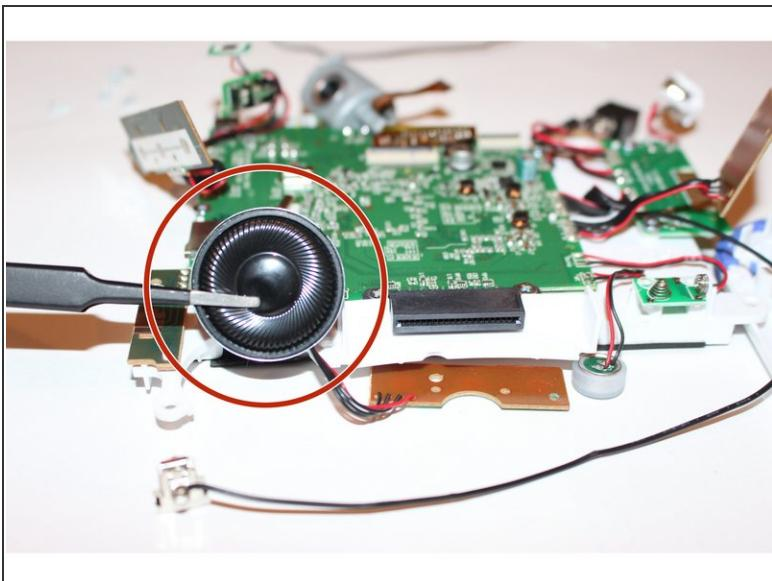
*(i)* The speakers are located in the bottom left of the device, and is shaped like a large black circle
