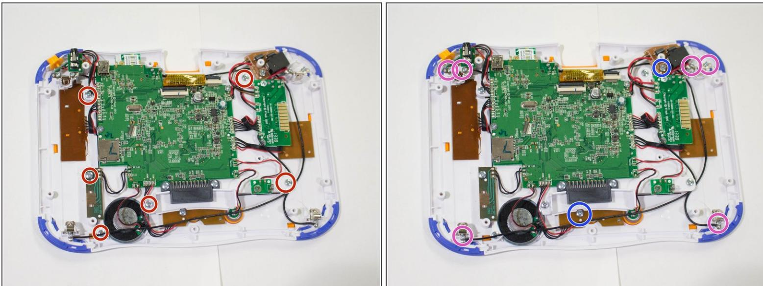
*(i)* There are six 5mm screws securing the motherboard to the front panel of the device.
