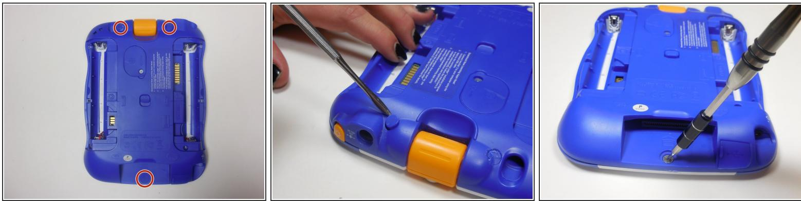
*(i)* There are three hidden screws on the back of the device, two at the top and one near the bottom.
