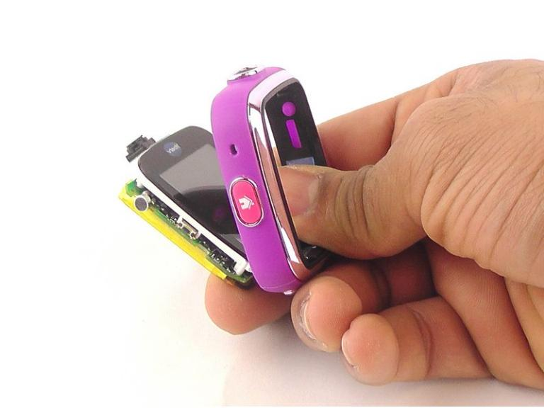
***i*** The speaker wires are fragile. They may break if excessive force is used to remove the circuit board.
