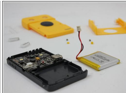
**⚠** Pull out the connector, be careful and only pull the connector and not the wires to avoid damaging them in the process.
