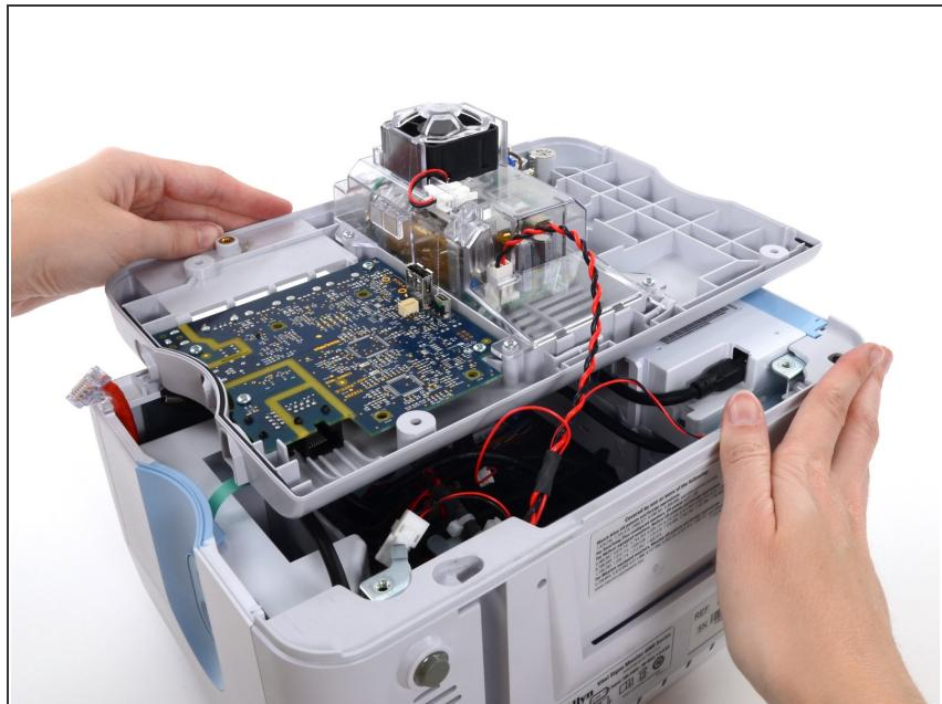
*(i)* The following connector requires two hands to disconnect. Flip the rear case over, and lay it on its back to gain access to the power supply cable.
