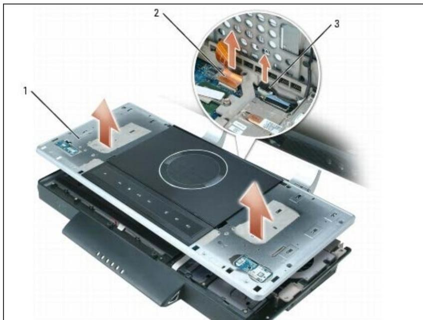
*(i)* Slightly lift up the top cover, but do not fully remove it. Two cables are connected to the top cover, and they could be damaged if the top cover is improperly removed.
