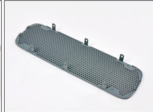
*(i) In the next few steps, you will use the tip of a spudger or the finger of an Xbox 360 opening tool to release the clips along the left and right sides of the bottom vent. Their locations are highlighted in red.*
