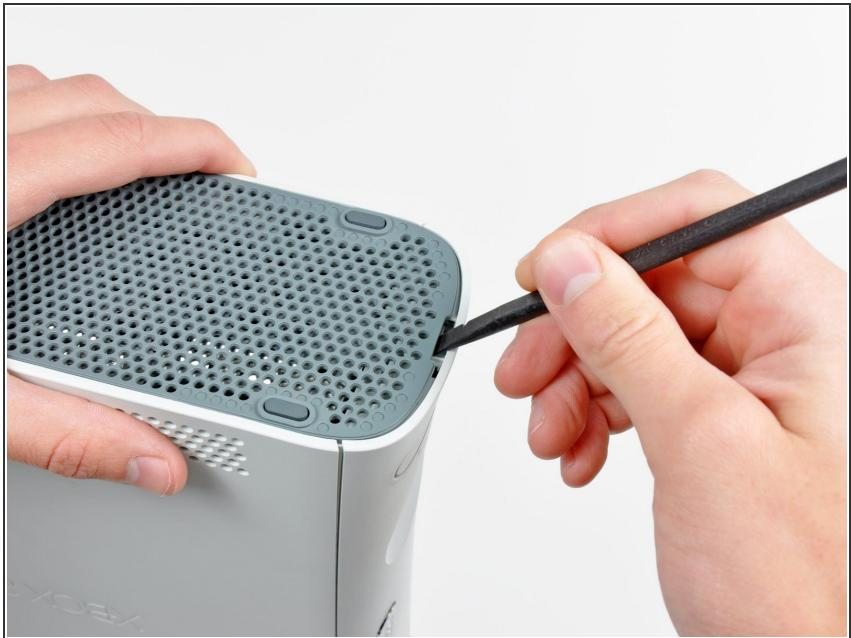
Stand the console vertically with the bottom edge facing up.
