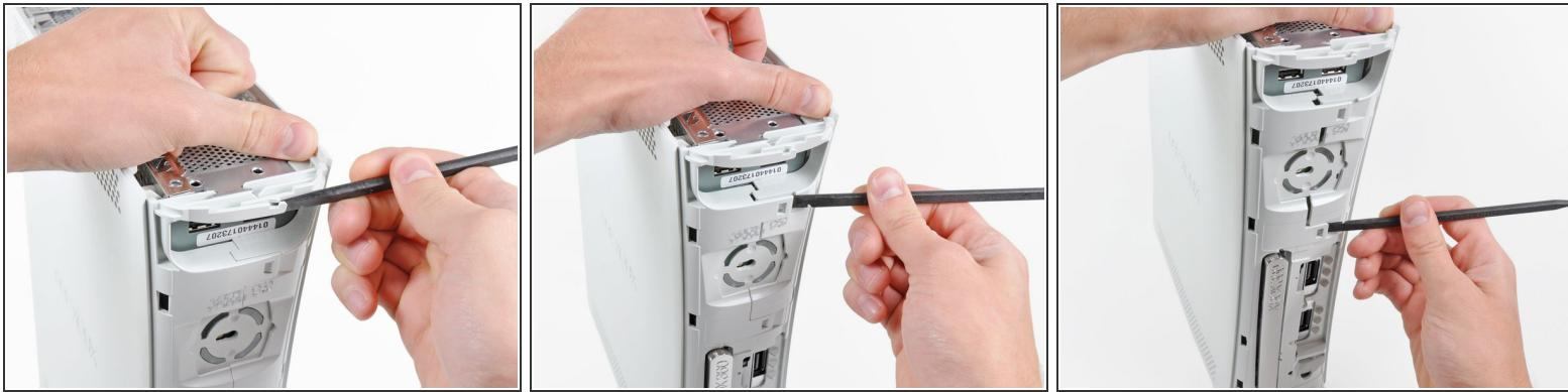
*(i)* The upper and lower cases are attached via several latches, located in the front and back of the console. These latches must be disengaged to separate the upper case from the console.
