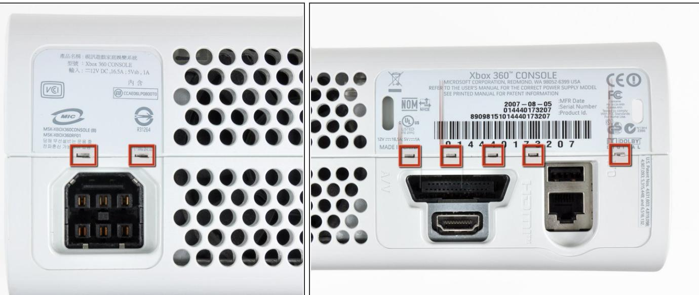
ⓘ The upper and lower cases are held together by seven release latches located on the back of the console. Their locations are highlighted in red.
