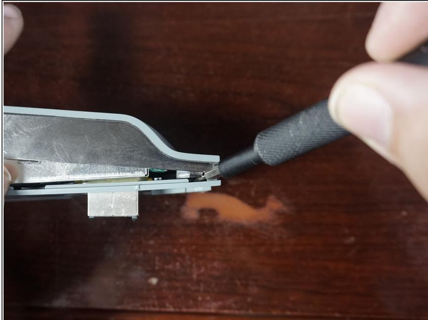
**★** If your drive is difficult to open, a screwdriver or plastic pry tool can be used to help open the enclosure.
