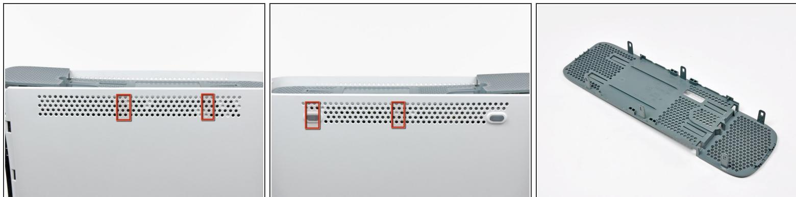
ⓘ In the next few steps, you will use the tip of a spudger or the finger of an Xbox 360 opening tool to release the clips along the left and right sides of the top vent. Their locations are highlighted in red.
