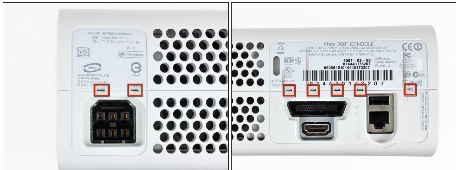
**i** The upper and lower cases are held together by seven release latches located on the back of the console. Their locations are highlighted in red.
