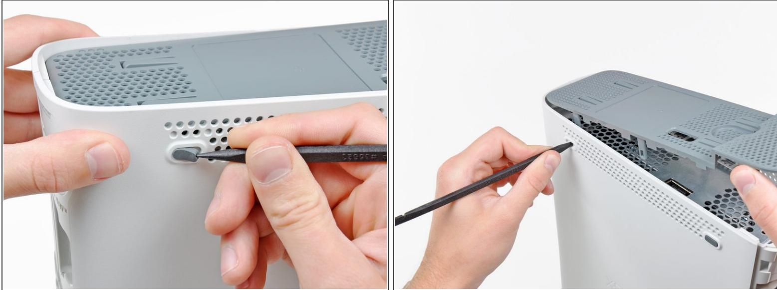
*(i)* The last clip is hidden underneath the rubber foot nearest the back of the console.
