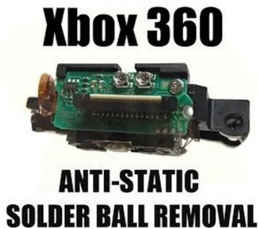
⚠ For a new laser lens that comes with an anti-static solder joint consult the video guide to remove the solder joint.
