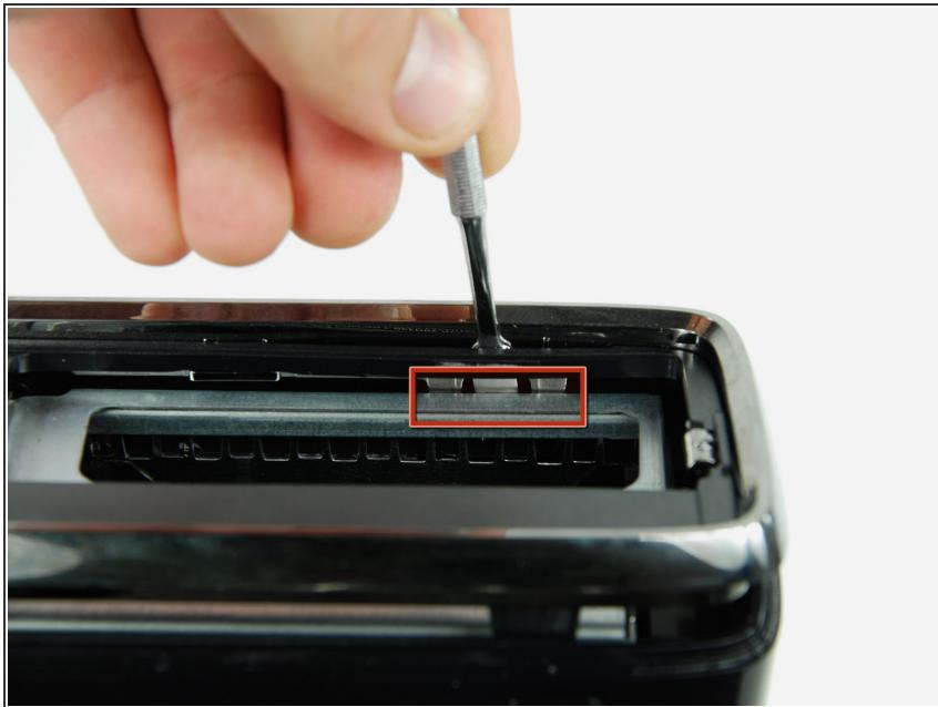
**i** This clip does not have a slit in the bezel to guide you. You can locate the clip by looking under the bezel near the hard drive slot.
