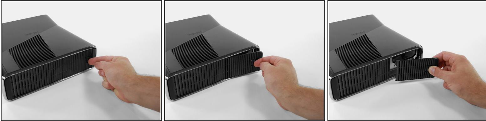
*(i)* Orient the Xbox 360 S so that the bottom of the console is facing toward you.
