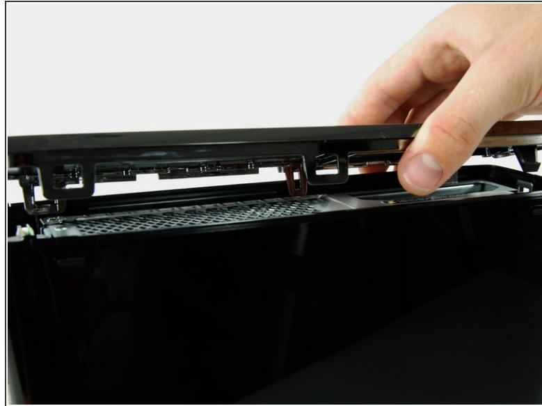
**i** This clip is smaller than the others and should not be removed from above like the others.
