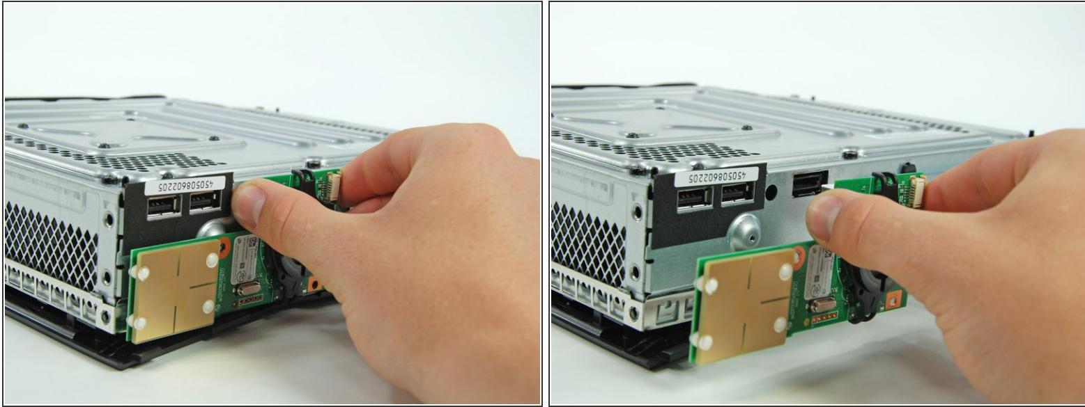
*(i)* The RF module is still connected to the Xbox by a large USB-type connector.
