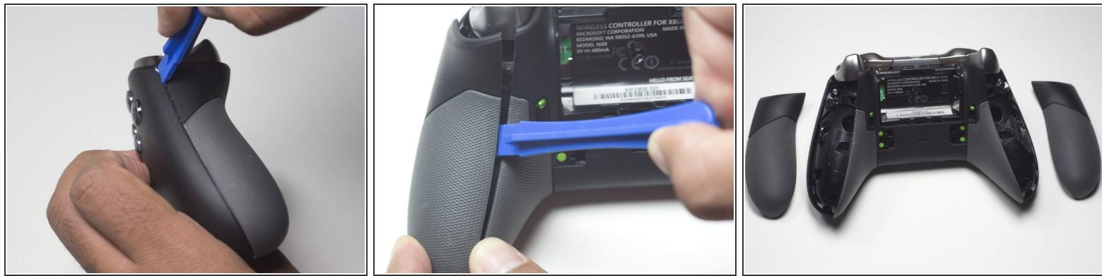
⚠ Be careful not to break the plastic tabs, that hold each grip cover to the back of the controller.
