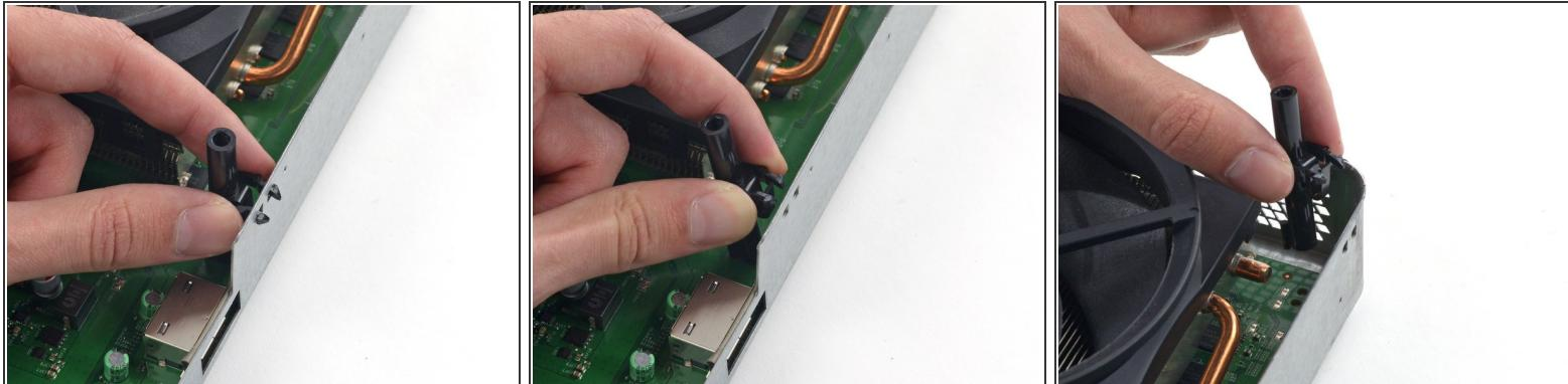
ⓘ Two black plastic screw posts are attached to the frame with springy plastic barbs.
