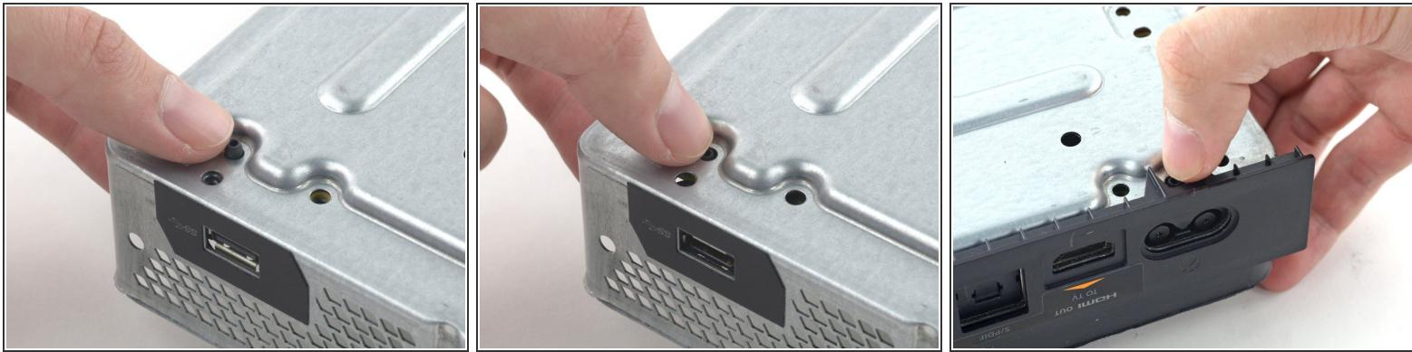
ⓘ Two small plastic plugs protrude through the rear metal case—one beneath the side USB port, and another beneath the AC in port. These plugs get caught on the lower metal case and make it hard to remove the motherboard.
