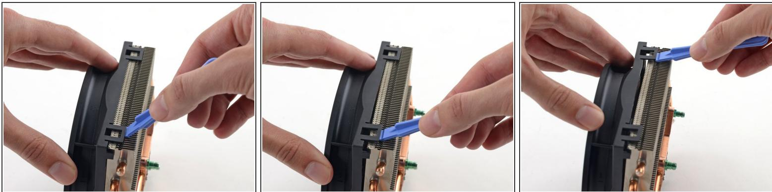
ⓘ The fan is held onto the heat sink with four sturdy plastic clips.
