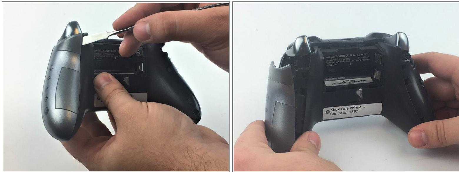
*(i)* We recommend using a plastic spudger to prevent damage to your controller. However, using a metal spudger, as shown in the picture, makes the work easier.
