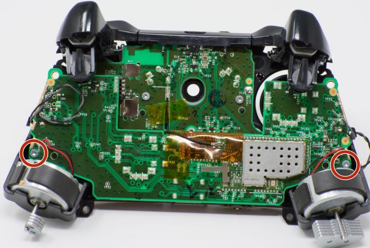
**⚠** If the rumble motors fall out of frame, the wires may disconnect from the motherboard. The wires will have to be soldered to reattach the motor.
