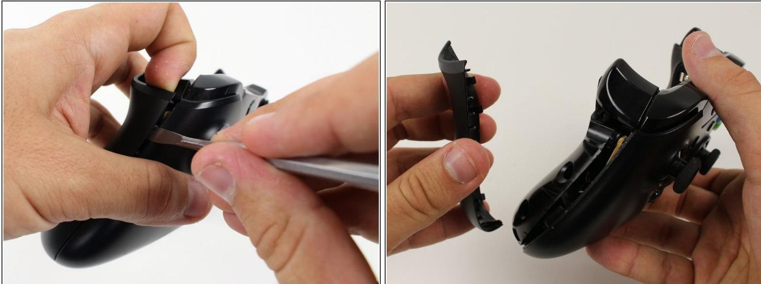
*(i)* We recommend using a nylon spudger for this step. A metal spudger is shown.
